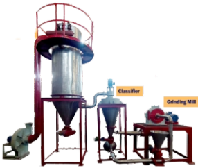
Universal Mill Fineness upto 5 microns
