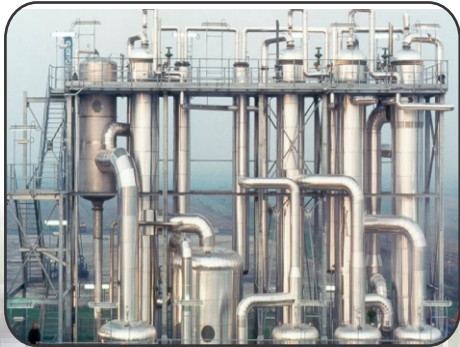
MULTIPLE EFFECT EVAPORATOR
